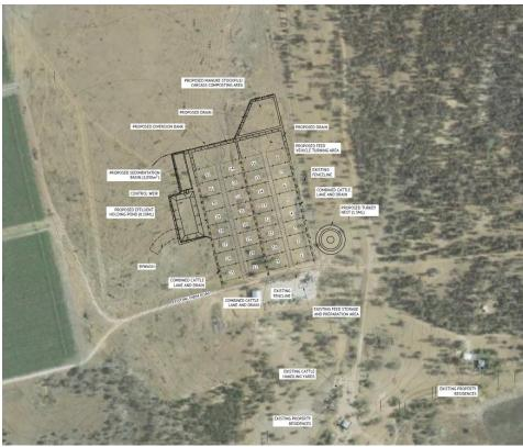
Figure 1: Feedlot development concept plan
