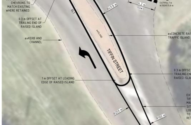
TIFFIN STREET / McDOWALL STREET INTERSECTION SCALE - 1:100
